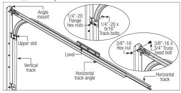
Next level the horizontal track assembly and bolt the horizontal track angle to the first encountered slot in the flag angle / angle mount using (1) 3/8" -  $16 \times 3/4$ " truss head bolt and (1) 3/8" - 16 hex nut. Repeat for other side. Remove nail that was temporally holding the top section in position.
