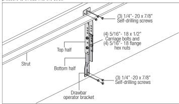
**B:** Locate the center of the top section. Position the drawbar operator bracket under the strut (if applicable) or align the drawbar operator bracket top edge with the top edge of the top section, as shown.
