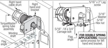
**FOR SINGLE SPRING APPLICATIONS:** Secure the idler bracket to the flag angle using (1) 5/16" -  $18 \times 3/4$ " carriage bolt, (1) 5/16" washer and (1) 5/16" -  $18 \times 3/4$ " carriage bolt, (1) 5/16" washer and (1) 5/16" -  $18 \times 3/4$ " carriage bolt, (1) 5/16" x 2" lag screw.
