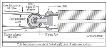
**NOTE:** Some larger doors feature 2 pairs of extension springs. A spring restraint cable must be installed through each spring.
