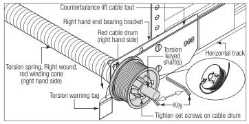
**IMPORTANT:** CHECK EACH COUNTERBALANCE LIFT CABLE, MAKING SURE BOTH ARE SEATED PROPERLY ON THE SHEAVES, CABLE DRUMS, ARE SECURELY ATTACHED TO THE BOTTOM CORNER BRACKETS AND BOTH SIDES HAVE EQUAL COUNTERBALANCE LIFT TENSION.
