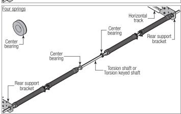
**IF YOU HAVE TWO TORSION KEYED SHAFTS:** With assistance, pick up the left hand torsion spring assembly and slide one end of the torsion keyed shaft through the end bearing bracket and loosely attach the oval bearing to the center bracket with (2) 3/8" - 16 x 1-1/2" hex head bolts and (2) 3/8" - 16 hex nuts, as shown. Repeat for others, if needed.
