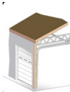
Low Headroom rear mount torsion
