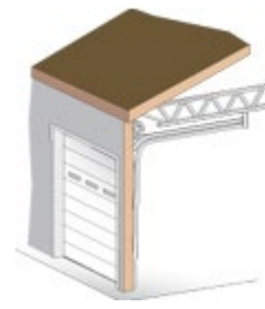
Low Headroom front mount torsion
