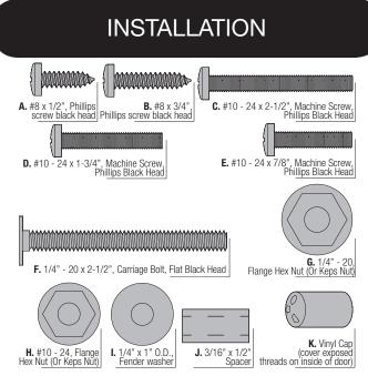
FOR FENDER WASHERS: (For use with vinyl-back insulated and paper-back insulated doors.)
