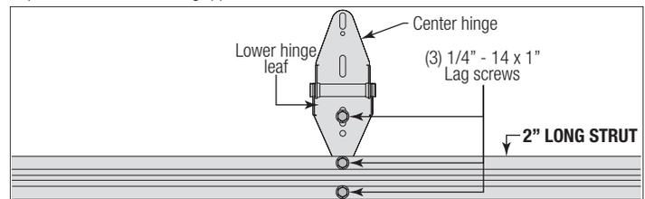
**IF YOU HAVE 3" LONG STRUTS:** Attach the upper leg of the strut to the upper slot of the center hinge using (1) strut clip and a 1/4" - 14 x 1" lag screw. Secure the lower leg of the strut to the hole of the center hinge using a 1/4" - 14 x 1" lag screw. Repeat for other center hinge(s).
