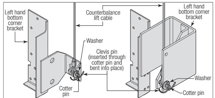
Locate the left hand bottom corner bracket. Align the bottom corner bracket horizontally with the bottom edge of the bottom section and also align the bottom corner bracket vertically with the left bottom edge of the bottom section. Mark and pre-drill 9/32" diameter holes through the bottom section. Attach the bottom corner bracket to the bottom section using (3) 1/4" - 20 x 2-1/4" carriage bolts and (3) 1/4" - 20 RED HEAD flange hex nuts. Repeat the same process for the right hand side.
