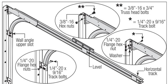
Next level the horizontal track assembly and bolt the top rail of the horizontal track to the encountered slot in the flag angle / angle mount using (1) 1/4" - 20 x 9/16" track bolt, (1) 1/4" - 20 flange hex nut and (1) 5/16" washer.
