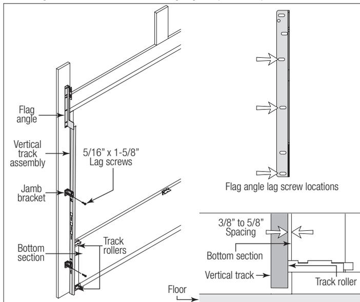
**FOR RIVETED VERTICAL TRACK ASSEMBLY:** Loosely fasten jamb brackets and flag angle to the jamb using 5/16" x 1-5/8" lag screws. Tighten lag screws, securing the bottom jamb bracket to jamb, maintain 3/8" to 5/8" spacing, between the bottom section and vertical track. Hang counterbalance lift cable over flag angle. Repeat same process for other side.
