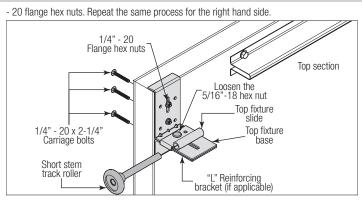
IF YOU HAVE FOUR TOP FIXTURE ASSEMBLIES: Position the second top fixture assembly next to the first installed top fixture assembly. Using the top fixture base as a template, drill pilot holes, 1" deep into the top section with a 1/8" drill bit (if needed).
