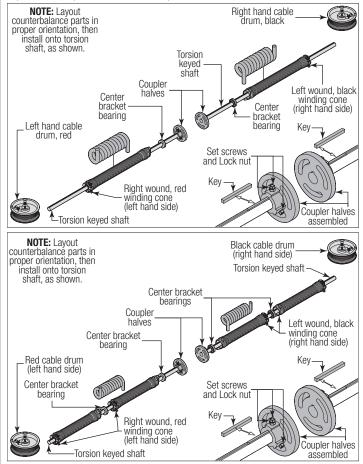
With assistance and starting on the left hand side of door, pick up the left hand torsion spring assembly and slide one end of the torsion keyed shaft through the end bearing bracket. Lay the other side of the torsion keyed shaft into the center bracket. Repeat the same process for the right hand torsion spring assembly.
