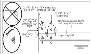
**IMPORTANT:** PUSH & HOLD THE HINGE LEAFS SECURELY AGAINST THE SECTIONS WHILE SECURING WITH APPROPRIATE FASTENERS. THERE SHOULD BE NO GAP BETWEEN THE HINGE LEAFS AND THE SECTIONS.
