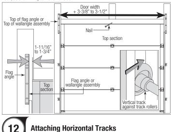
**NOTE:** Depending on your door, you may have Fully Adjustable Flag Angles, Riveted Vertical Track Assemblies or you may have Angle Mount Vertical Track Assemblies. Refer to Package Contents / Breakdown of Parts, to determine which Flag Angles / Vertical Track Assemblies you have.
