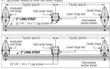
If you have single graduated end hinges, insert a short stem track roller / short stem tandem track roller (if included) into the hinge tube on each side.
