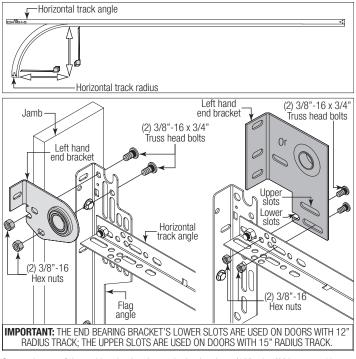
Secure the top of the end bearing bracket to the jamb using  $5/16" \times 1-5/8"$  lag screw(s). Repeat the same process for right hand side.
