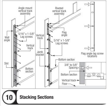
NOTE: Refer to door section identification, located in the pre-installation section of this
