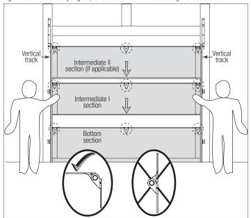
FOR CENTER HINGE(S) AND OR HALF CENTER HINGE(S): Flip a upper hinge leaf up and use it as a template. Mark and pre-drill (2) 1/8" pilot holes, 1" deep into the section with a 1/8" drill bit.
