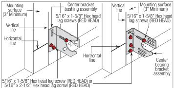
IF YOUR DOOR DID COME WITH A CENTER COUPLER ASSEMBLY OR 3-3/4" ID TOR-SION SPRINGS: Mark a vertical pencil line on the mounting surface above the door, at the center. Split the difference up and position the (2) center bearing brackets apart from each other. Mark two vertical pencil lines, one for each center bearing bracket onto the mounting surface above the door.
