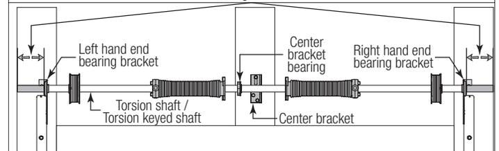
**IF YOU HAVE A COUPLER ASSEMBLY:** Disassemble the coupler assembly by removing the (3) 3/8" - 16 x 1-1/2" hex head screws, (6) 3/8" washers, (3) 3/8" lock washers and the (3) 3/8" - 16 hex nuts from the coupler halves. Loosen the set screws. Set the components aside.
