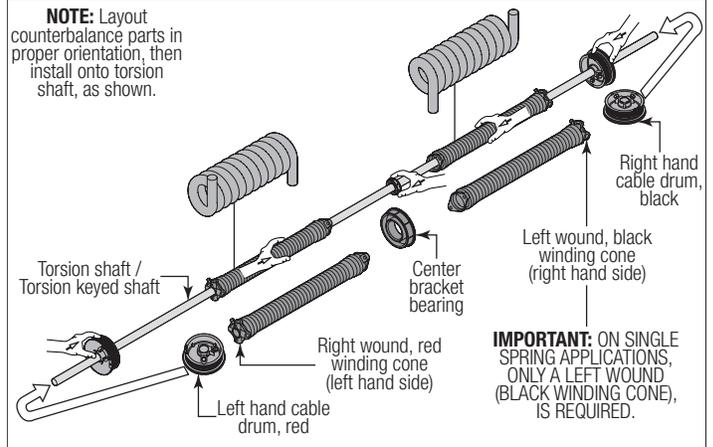
With assistance, pick up the torsion spring assembly and slide one end of the torsion shaft / torsion keyed shaft through one end bearing bracket. Lay the middle of the torsion shaft / torsion keyed shaft into the center bracket. Slide the other end of the torsion shaft / torsion keyed shaft into the other end bearing bracket.
