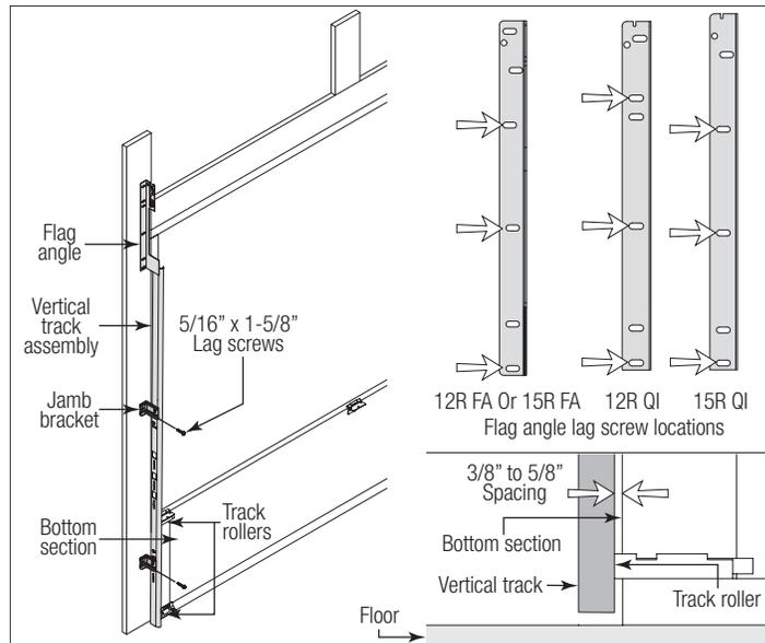
**FOR RIVETED VERTICAL TRACK ASSEMBLY:** Loosely fasten jamb brackets and flag angle to the jamb using 5/16" x 1-5/8" lag screws. Tighten lag screws, securing the bottom jamb bracket to jamb, maintain 3/8" to 5/8" spacing as shown between the bottom section and vertical track. Hang counterbalance lift cable over flag angle. Repeat same process for other side.
