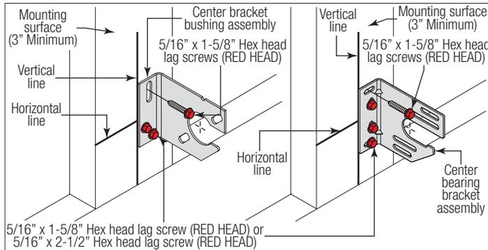
**IF YOUR DOOR DID COME WITH A CENTER COUPLER ASSEMBLY OR 3-3/4" ID TORSION SPRINGS:** Mark a vertical pencil line on the mounting surface above the door, at the center. Split the difference up and position the (2) center bearing brackets apart from each other. Mark two vertical pencil lines, one for each center bearing bracket onto the mounting surface above the door.
