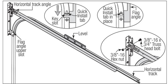
**FOR OTHER FLAG ANGLES:** To install horizontal track, place the curved end over the top track roller of the top section. Align the bottom of the horizontal track with the top of the vertical track. Tighten the horizontal track to the flag angle with (2) 1/4" - 20 x 9/16" track bolts and (2) 1/4" - 20 flange hex nuts.
