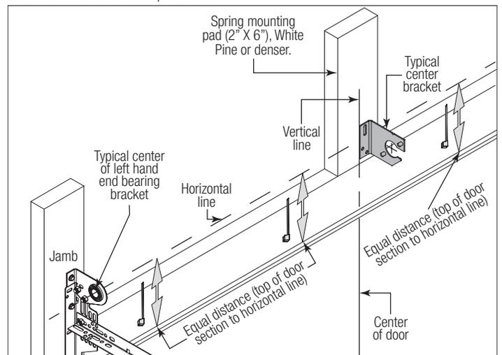
**IF YOUR DOOR DID NOT COME WITH A CENTER COUPLER ASSEMBLY OR TORSION SPRINGS LESS THAN 3-3/4" ID:** Mark a vertical pencil line on the mounting surface above the door, at the center. Align the edge of the center bracket with the vertical pencil line and the center of the center bracket with the horizontal pencil line; this is to ensure the torsion shaft is level between the center and end bearing brackets.
