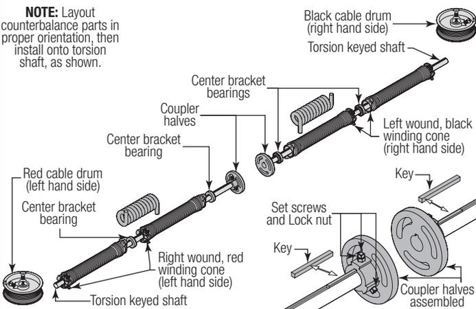
With assistance and starting on the left hand side of door, pick up the left hand torsion spring assembly and slide one end of the torsion keyed shaft through the end bearing bracket. Lay the other side of the torsion keyed shaft into the center bracket. Repeat the same process for the right hand torsion spring assembly.
