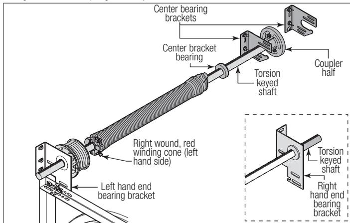
**NOTE:** Position both torsion keyed shafts so that equal amounts of the shafts extend from each end bearing brackets.
