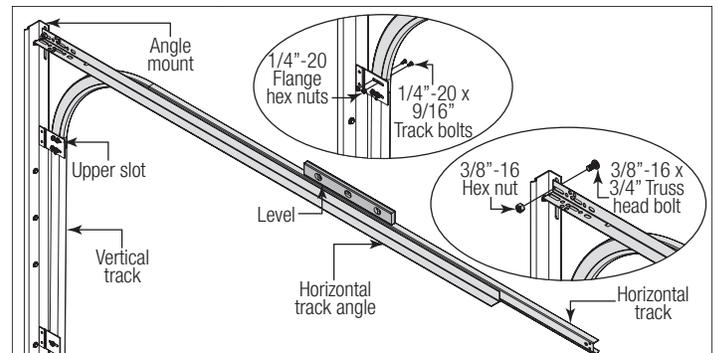
Next level the horizontal track assembly and bolt the horizontal track angle to the first encountered slot in the flag angle / angle mount using (1) 3/8" - 16 x 3/4" truss head bolt and (1) 3/8" - 16 hex nut. Repeat for other side. Remove nail that was temporarily holding the top section in position.
