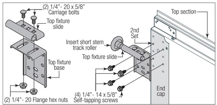
**IF YOU HAVE TOP FIXTURE ASSEMBLIES:** Starting on the left hand side of the top section, place the top of the top fixture base flush with the top edge of section and even with the edge of the endcap. Fasten the top fixture assembly to the top section using (4) 1/4" - 20 x 7/8" self drilling screws. Next, loosen the 5/16" - 18 hex nut on the 5/16" - 18 x 5/8" carriage bolt. Insert short stem track roller into top fixture slide. Repeat the same process for the right hand side.
