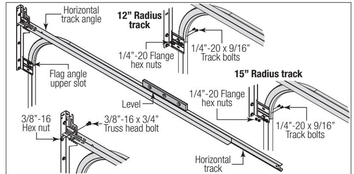
**IF YOU HAVE ANGLE MOUNT:** To install horizontal track, place the curved end over the top track roller of the top section. Align the bottom of the horizontal track with the top of the vertical track. Tighten the horizontal track to the angle mount with (2) 1/4" - 20 x 9/16" track bolts and (2) 1/4" - 20 flange hex nuts.
