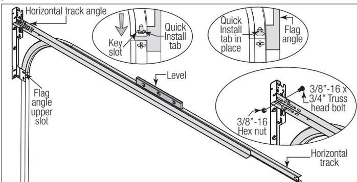
**FOR OTHER FLAG ANGLES:** To install horizontal track, place the curved end over the top track roller of the top section. Align the bottom of the horizontal track with the top of the vertical track. Tighten the horizontal track to the flag angle with (2) 1/4" - 20 x 9/16" track bolts and (2) 1/4" - 20 flange hex nuts.
