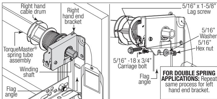
**FOR SINGLE SPRING APPLICATIONS:** Secure the idler bracket to the flag angle using (1) 5/16" - 18 x 3/4" carriage bolt, (1) 5/16" washer and (1) 5/16" - 18 hex nut. Then secure the idler bracket to the jamb using (1) 5/16" x 1-5/8" lag screw.
