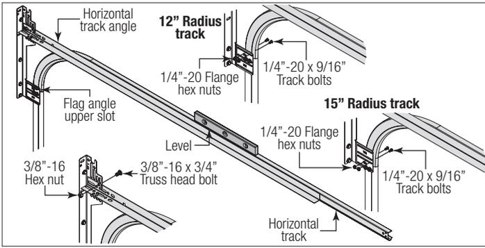
Next level the horizontal track assembly and bolt the horizontal track angle to the first encountered slot in the flag angle / angle mount using (1) 3/8" - 16 x 3/4" truss head bolt and (1) 3/8" - 16 hex nut. Repeat for other side. Remove nail that was temporarily holding the top section in position.
