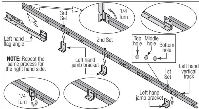
**FOR DOORS WITH FULLY ADJUSTABLE TRACK:** Hand tighten the left hand flag angle to the left hand vertical track using (2) 1/4" - 20 x 9/16" track bolts and (2) 1/4" - 20 flange hex nuts.
