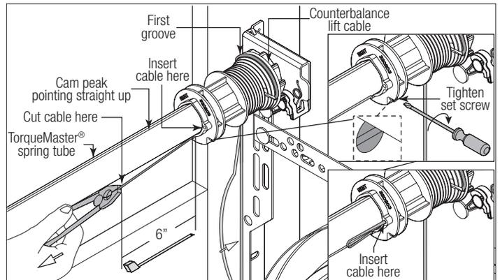
**NOTE:** Illustration shows the right hand cable drum assembly. Repeat the same process for the left hand side.
