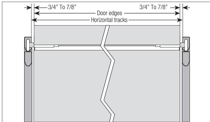
Remove any locking pliers. Lift the door and check its balance. Adjust spring(s) if door lifts by itself (hard to pull down) or if door is difficult to lift (drifts down). Anytime spring adjustments are made, ratchet pawl knob must be in the upper position. An unbalanced door can cause TorqueMaster® Plus operation problems.
