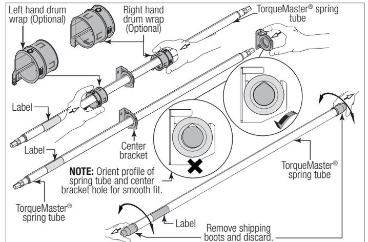
**12 Installing Cable Drum Assemblies**
