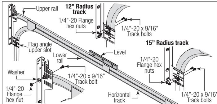
Next level the horizontal track assembly and bolt the top rail of the horizontal track to the encountered slot in the flag angle using (1) 1/4" - 20 x 9/16" track bolt, (1) 1/4" - 20 flange hex nut and (1) 5/16" washer. Repeat for other side.
