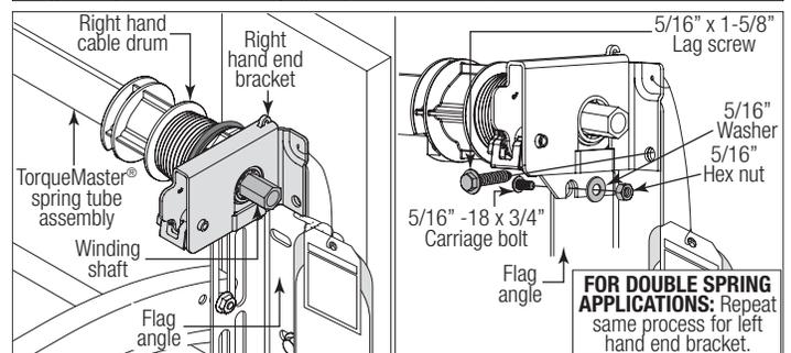
**FOR DOUBLE SPRING APPLICATIONS:** Repeat same process for left hand end bracket.
