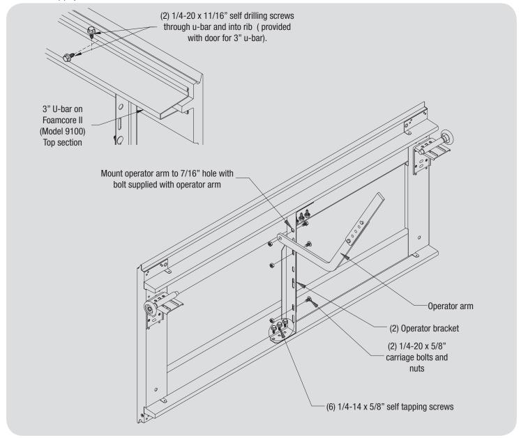
Align both pieces of the operator bracket between the ribs on the top section. Loosely assemble the brackets using (2)  $1/4-20 \times 5/8$ " carriage bolts and nuts. Attach the assembly at the center of the door section using (6)  $1/4-14 \times 5/8$ " self tapping screws. Tighten both  $1/4-20 \times 5/8$ " bolts. Attach operator arm to 7/16" hole at the upper end of the operator bracket assembly.
