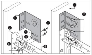
Figure 45, Left Side Shown (For L4. Bracket)
