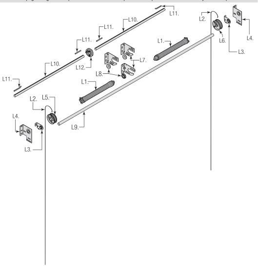
Figure 7 - Counterbalance Components
