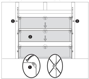
Figure 30, Stacking Sections
