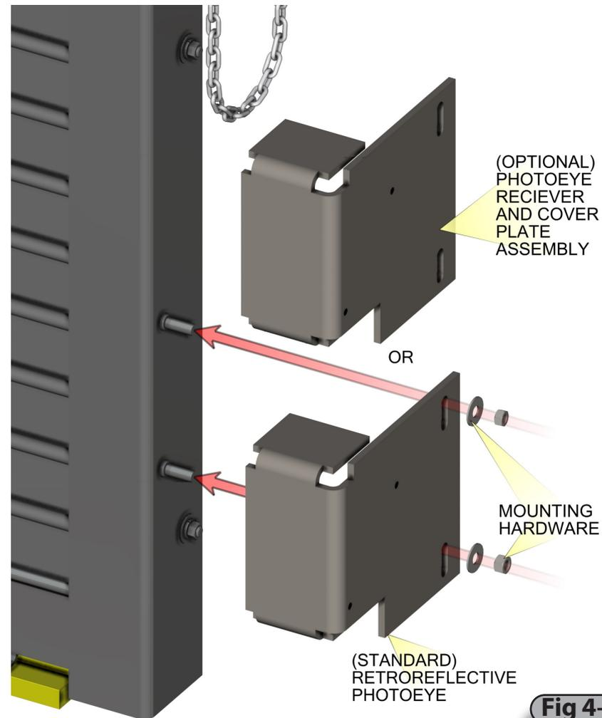
**NOTE:** Photoeyes are attached to their protective brackets at the factory and must be mounted to the guides using the hardware provided.
