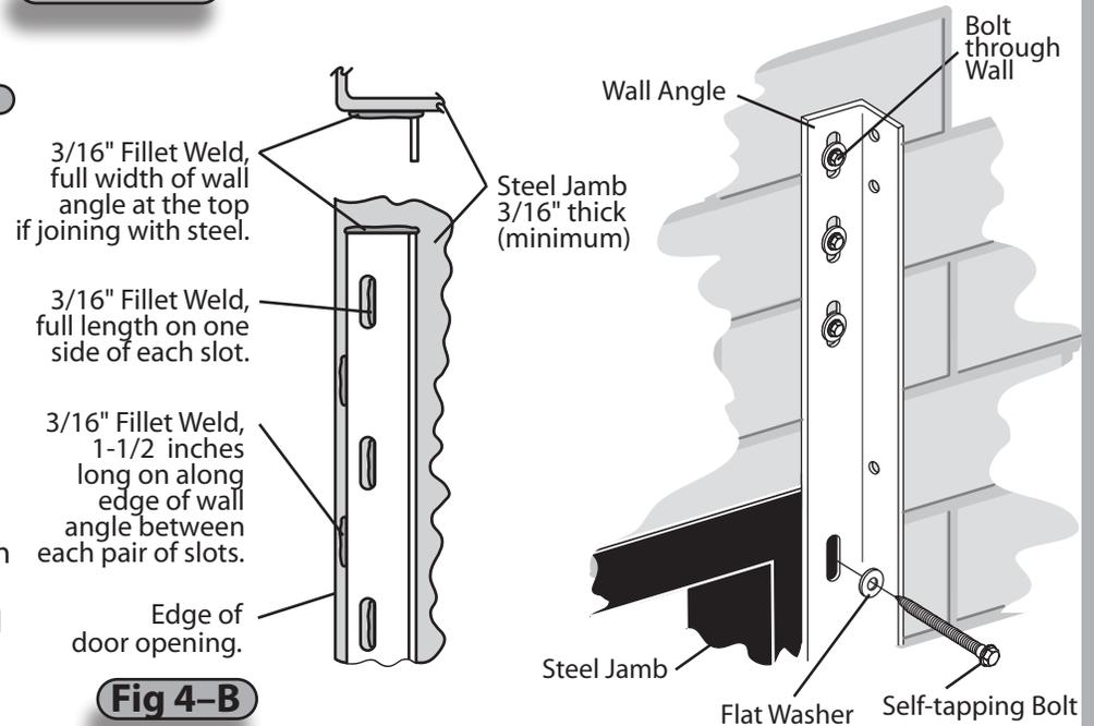
**NOTE:** When the wall angle extends above the steel of the jamb or header, use washers, spacers or shims to fill the gap between the masonry portion of the wall and the wall angle. Use through bolts to fasten the wall angle in the area above steel, **Fig. 4-C**.
