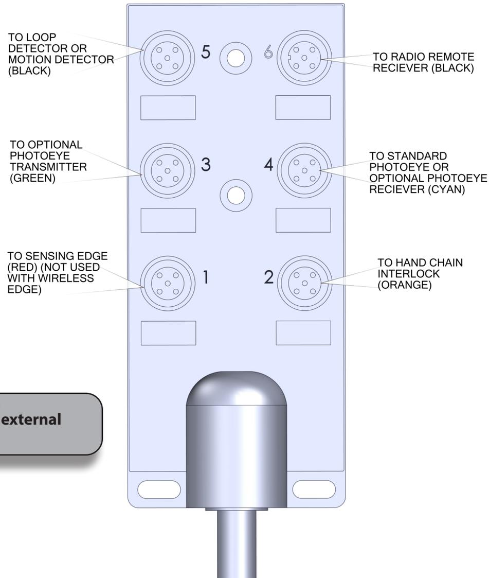
**Fig. 5-J JUNCTION BOX WIRING**
