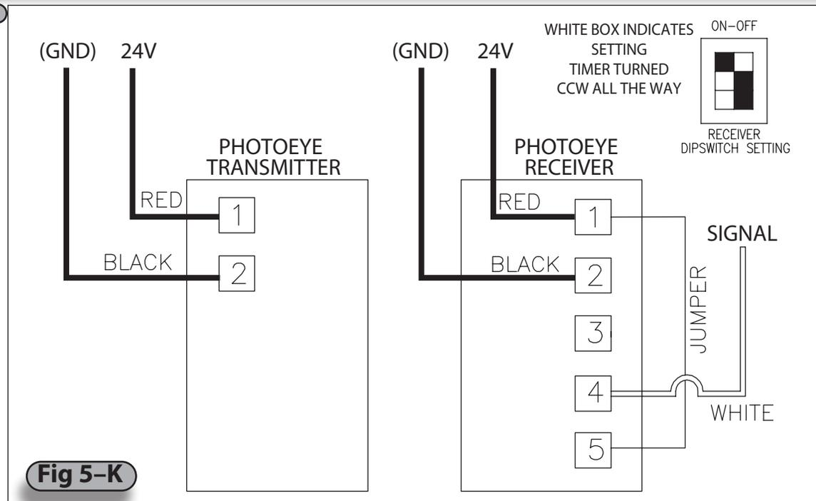
\* Photoeye cables are wired at the factory with a M12 connector. wire colors are for reference.
