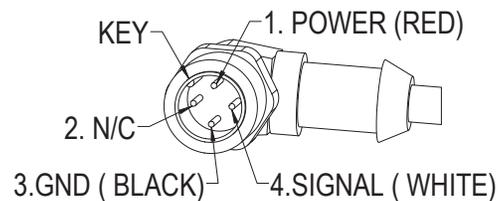
Photoeye Receiver Cable connects to Junction Box
