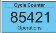
Cycle counter shows the number of operating cycles the door has completed (open/close = 1 cycle). Note: This is already shown by default at the top left corner in the main screen.
