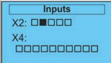
Inputs provides an overview of the controller inputs. Box is marked if the corresponding controller input is active.
