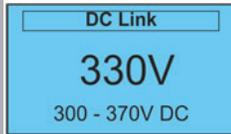
DC Link shows the internal DC Link voltage along with the acceptable range.
