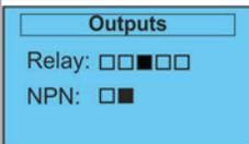
Outputs provides an overview of the controller outputs. Box is marked if the corresponding controller output is active.
