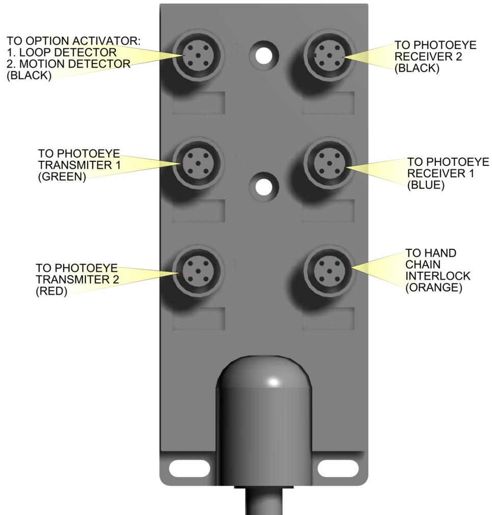
**Fig 19 JUNCTION BOX WIRING**
