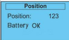
Position shows the internal door position count. The battery level and status are shown
