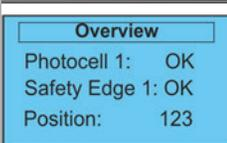
Overview displays status and current position of Photocell and Safety Edge (reversing edge)
