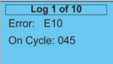
Fault log displays error code and door operation cycle for the last 10 faults. Scroll up or down to navigate through the fault log.
