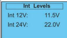
INT Levels shows the control's actual internal supply voltages.
