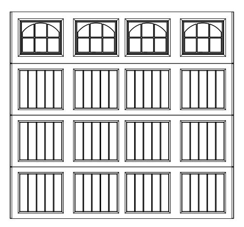
7'6" X 7' 9100/9605 SONOMA DESIGN 4 SECTION/4 PANEL CASCADE I TOP SECTION SHOWN CONSISTS OF (4) 20.8" SECTIONS
