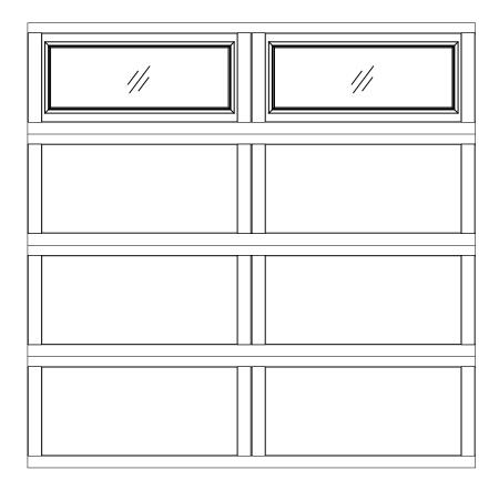
8 X 8 9405 WESTFIELD DESIGN 4 SECTION / 2 PANEL STYLELINE III TOP SECTION SHOWN CONSISTS OF (4) 23.8" SECTIONS
