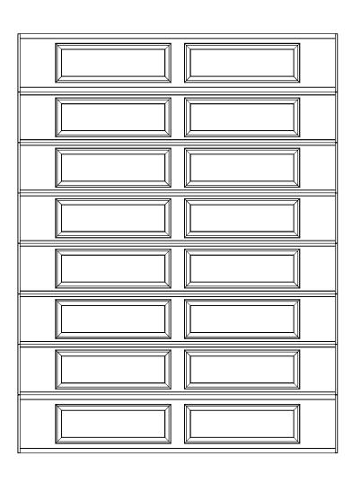
9'6" X 12'6" 8300/8500 ERP DESIGN 8 SECTION/ 2 PANEL SOLID TOP SECTION (6) 18" & (2) 20.8" SECTIONS
