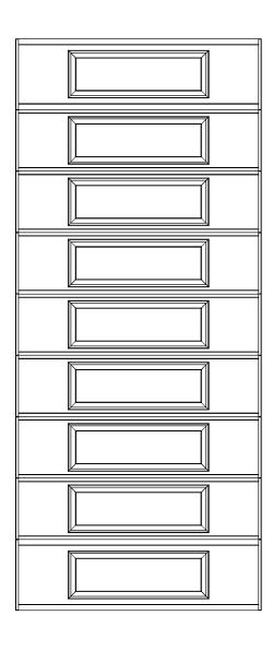
6'0" X 14'0" 8300/8500 ERP DESIGN 8 SECTION/ 1 PANEL SOLID TOP SECTION (7) 18" & (2) 20.8" SECTIONS
