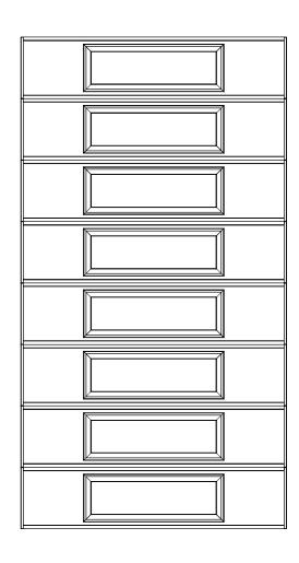
6'6" X 12'0" 8300/8500 ERP DESIGN 8 SECTION/ 1 PANEL SOLID TOP SECTION (8) 18" SECTIONS
