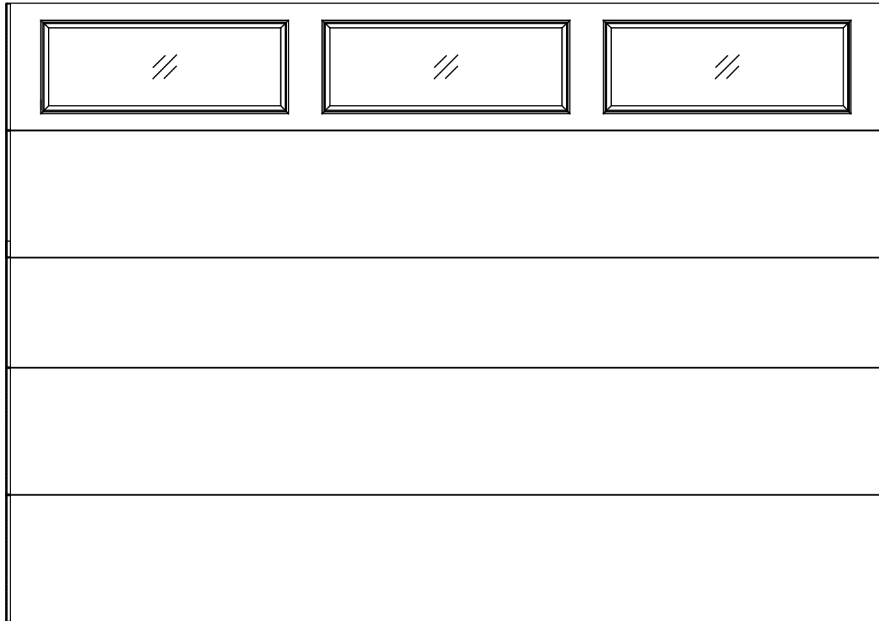
12'x8'6" 8300/8500 FLUSH DESIGN 5 SECTION/1 PANEL STYLELINE III TOP SECTION SHOWN (1) 18" & (4) 20.8" SECTIONS
