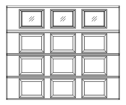
7'6"x6'3" 8300/8500 CRP 4 SECTIONS/ 3 PANELS STYLELINE I TOP SECTION SHOWN (3) 18.0" & (1) 20.8" SECTIONS
