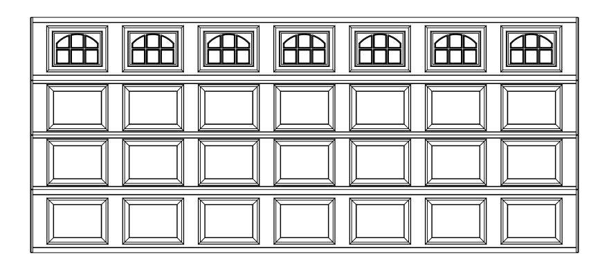
15'x6'6" 8300/8500 CRP 4 SECTIONS/ 7 PANELS CASCADE I TOP SECTION SHOWN (2) 18.0" & (2) 20.8" SECTIONS
